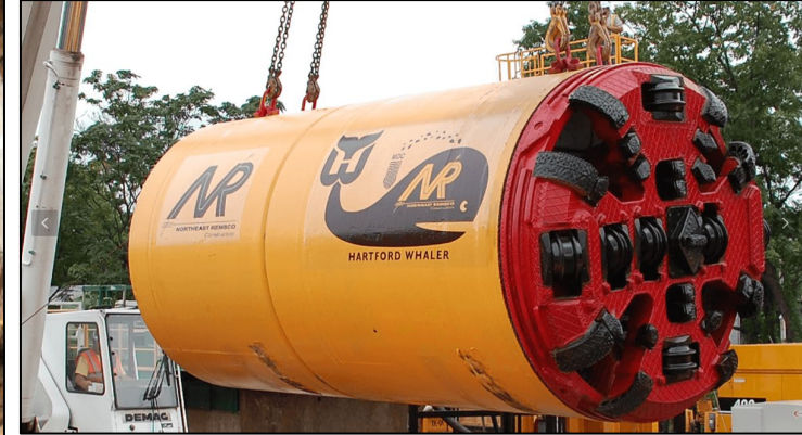
Microtunnel Boring Machine
