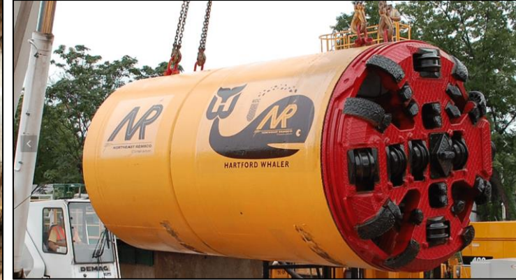
Microtunnel Boring Machine
